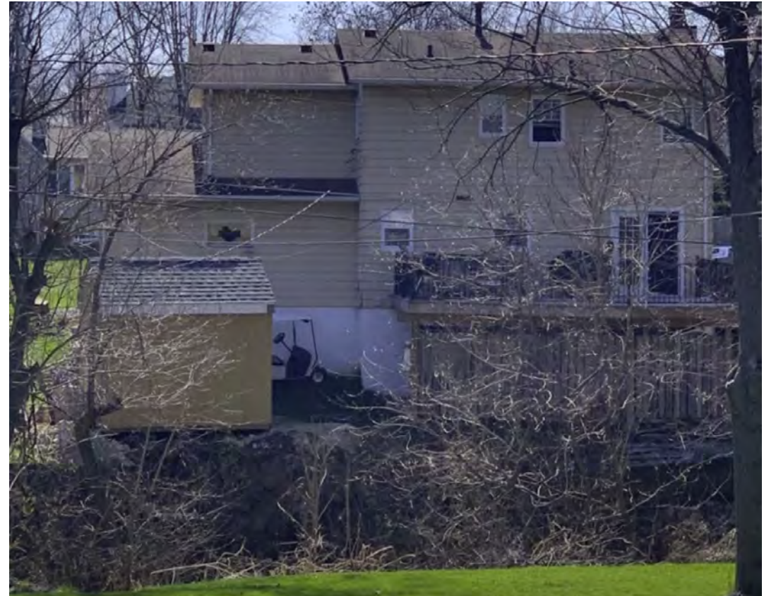
Figure 3.01-2.4: City staff noted that the small urban stream in this area was 2 feet wide and 1 foot deep when the area was platted about 30 years before this photo was taken. In this photo, the stream had a top width of around 40 feet and a depth of 15 feet.
