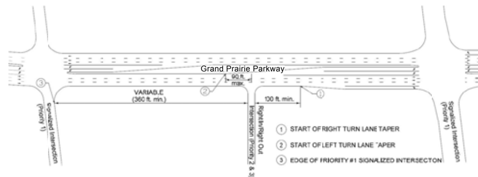
Figure 45-2: Right-In / Right-Out Location Criteria
