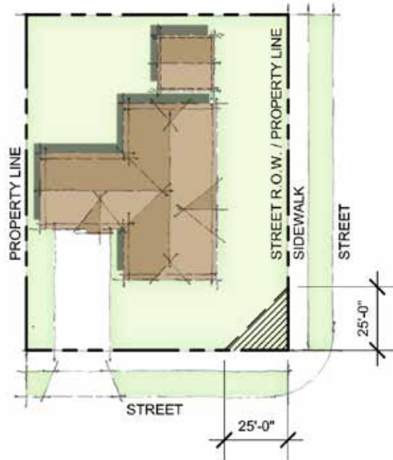
Figure 49-1: Intersection / Corner Lot Vision Clearance
